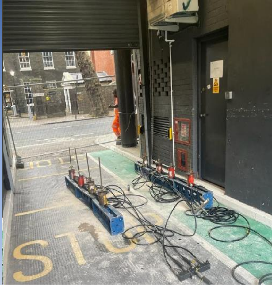
Photos of a test setup for the 21ton demolition excavator
