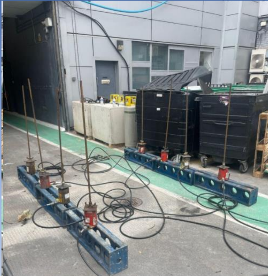
Photos of a test setup for the 21ton demolition excavator
